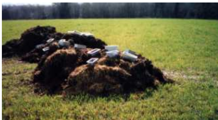
Figure 14: Measurement of N 2 O and CH 4 emissions during storage of cattle manure.
